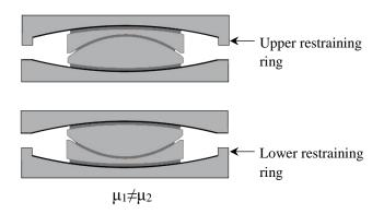
Figure 2. Double-surface friction pendulum isolators with unequal upper and lower surface friction coefficients.
