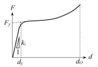
Figure 3. Force-displacement curve of metallic dampers with adaptive behavior.
