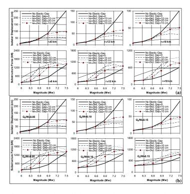
Figure 5: (a) Isolator displacement and SF versus ground motion magnitude for various fault
