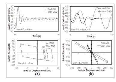
Figure 3: Comparison of the velocity time histories and isolator force- displacement hysteretic behaviors of a regular SIB and a SIB with EGD for NF ground motions with (a) Mw=6, r=6 km (b) Mw=7.5, r=6 km.
