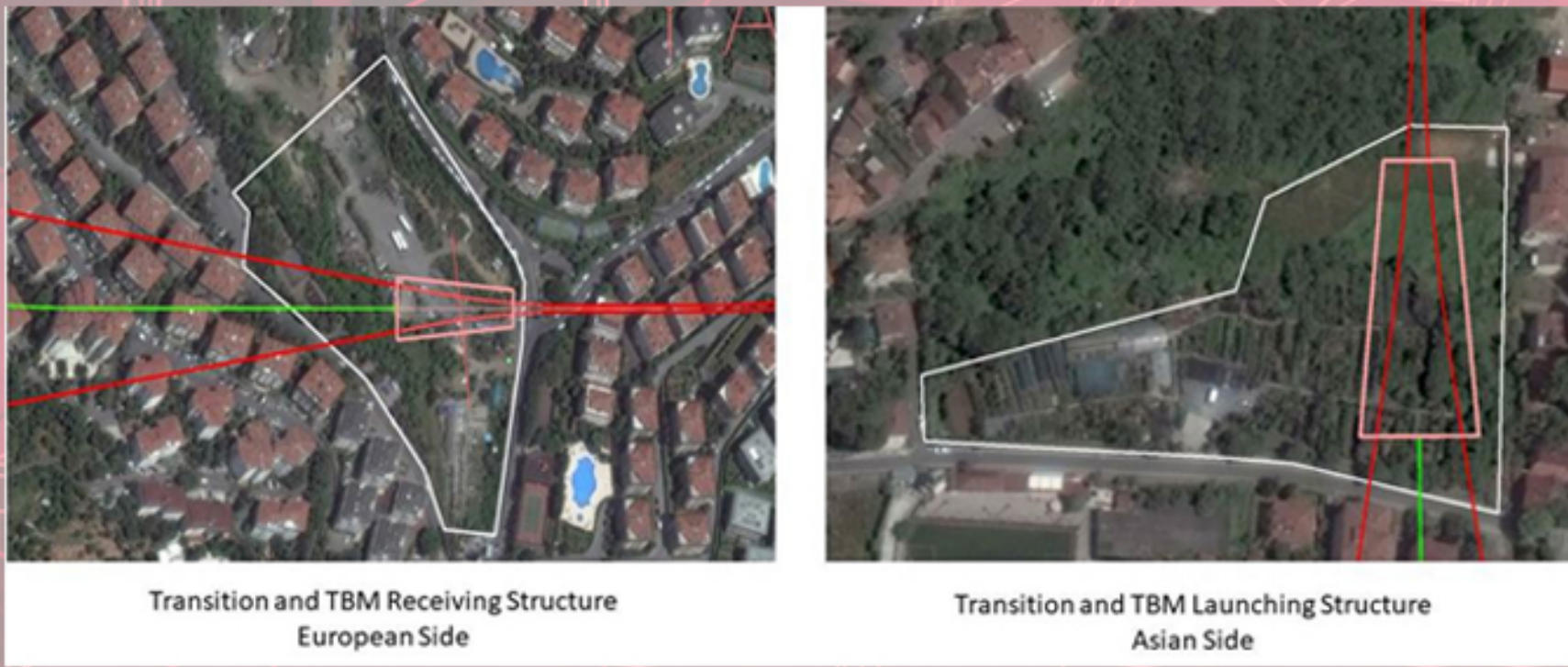
Figure 8 - Layout of Transition and TBM Launching and Receiving Structures
