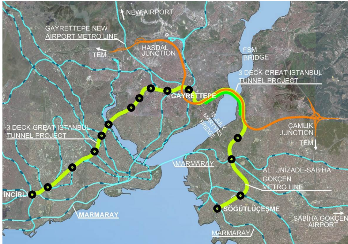
Figure 1 - 3-Deck Great Istanbul Tunnel Project both highway (orange line) and metro (yellow line) sections including combined Bosphorus crossing (green line) (author)
