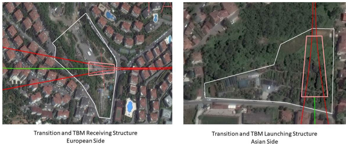
Figure 8 - Layout of Transition and TBM Launching and Receiving Structures (author)
