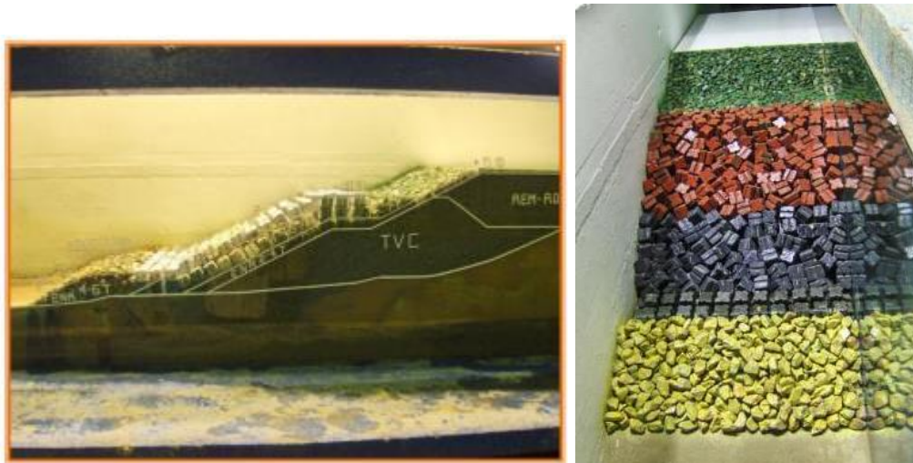
Figure 13: Suggested cross section of the revetment in laboratory conditions
