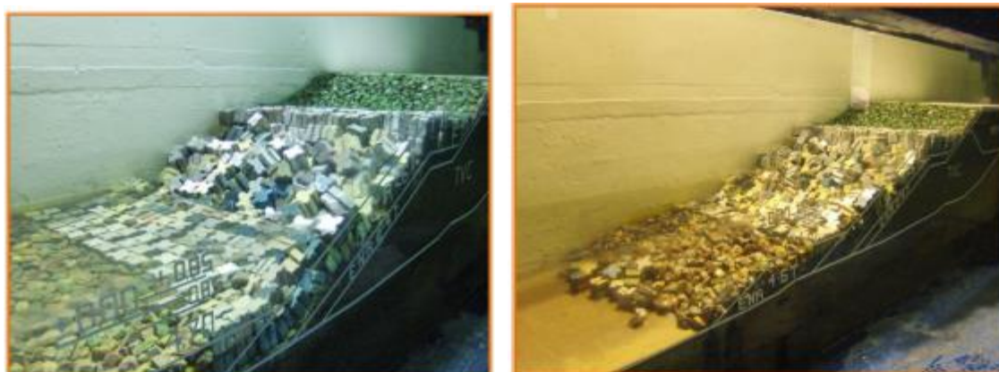
Figure 14: Damage of irregular placement of antifer block after a series of tests
