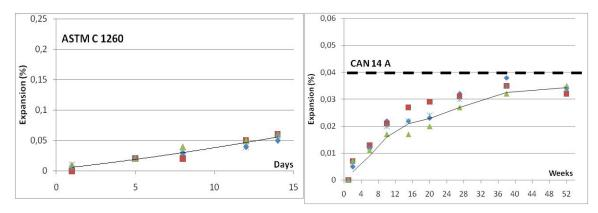
Figure 5. Expansion test results of crushed sand
