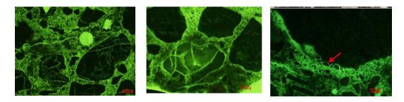
Figure 4. UV light views of reacted porous sandstone (left, x50), porous chert (middle, x100), biomicritic limestone with disseminated secondary microquartz (x50).
