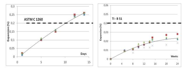
Figure 3. Expansion test results of natural sand
