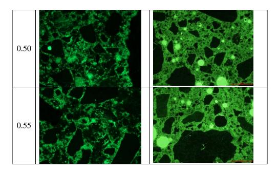
Fgure 2. Effect of water-to-cement ratio and cementitious material content on the UV light intensity under polarising microscope (x50).
