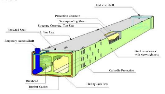
Figure 2. Typical Section View of Immersed Element
