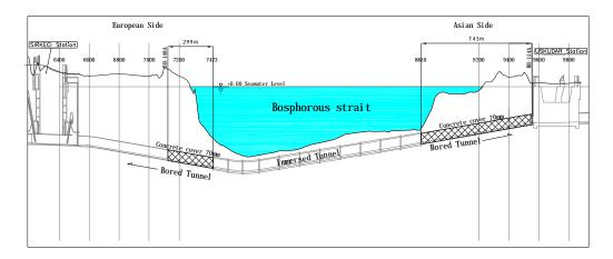
Figure 1. The range in which the concrete cover is 70 mm
