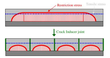
Figure 7. Effect of crack inducer joint
