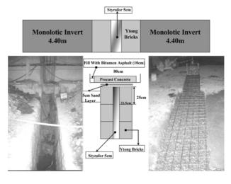
Figure 7. Detailed seismic joints in the monolithic invert.
