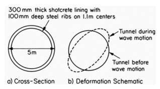
Figure 2. Picture during re-mining of Bench Pilot Tunnels (BPT) showing typical floor heave and buckled steel rib + shotcrete shell. (a-b) BPT Cross-Section and Seismic Distortion.
