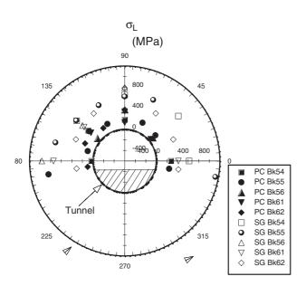
Figure 4. Earthquake induced radial stresses (kPa) on inner lining from pressure cells and embedded strain gauges.
